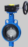
Butterfly Valves Wafer Type with Gearbox DN 50-600 mm PN 6-16 bar ANSI Class 150
